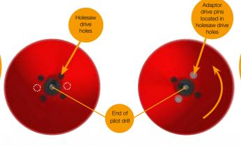
If the holesaw is turned in the direction of the arrow, the drive pins can be located in the first pair of drive holes they arrive at.
